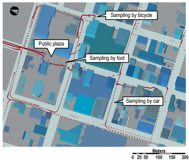
Figure 4. An example of signal sampling for a section of the Temple Square district. Roads are illustrated in light gray, with buildings represented in shades of blue. Darker gray areas are parcel boundaries, many of which represent the confines of public property. (The view in this figure is oblique, illustrating the relative heights of buildings, but this obscures some portions of adjacent sidewalks from which samples were obtained.)
